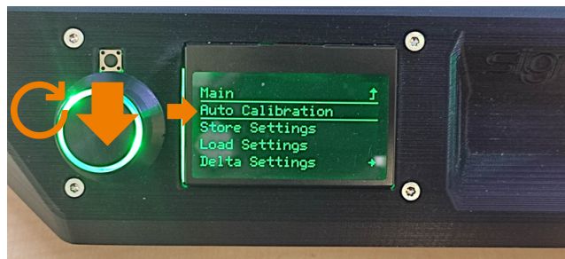
2 - Navigate downwards to 'Configuration' and press to confirm.
