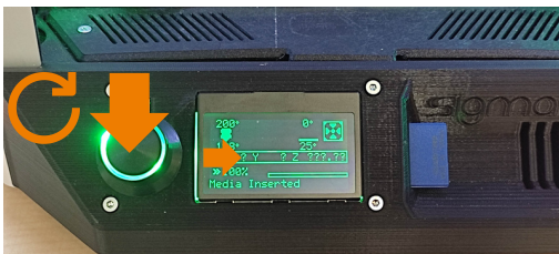
1 - Insert the SD card including the G-code
